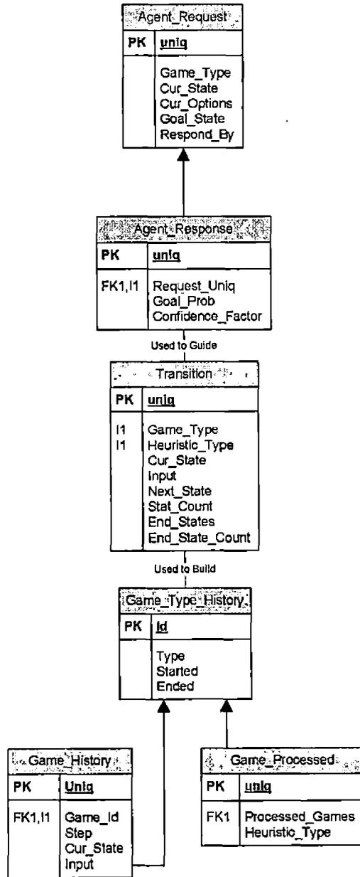
Fig. 3.3: FABLE Database Entity Relationship Diagram.
