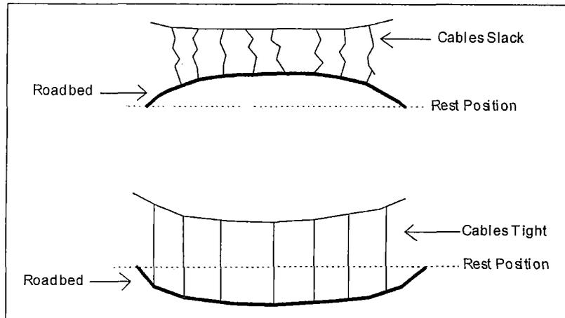
Figure 4. Bridge, Cables Tight and Slack
