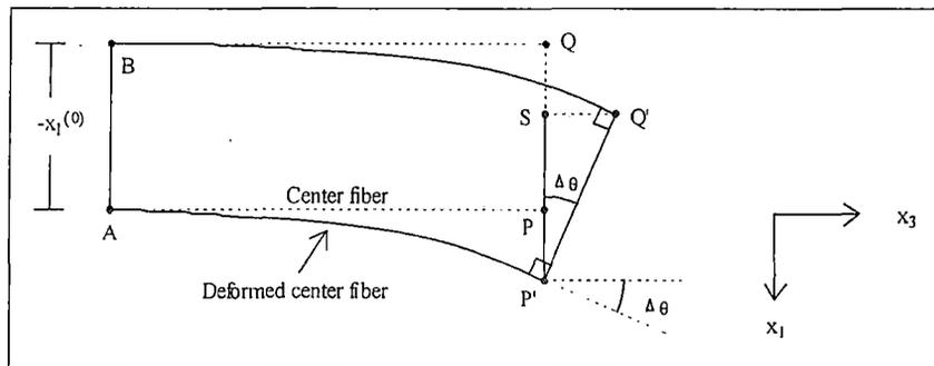
Figure 10. Beam Deformation
