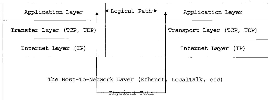
Figure 2.7. The Four-Layer Model of A Network
