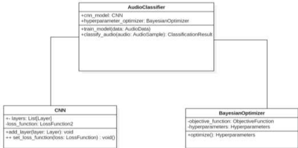
*Figure2. Class Diagram*
