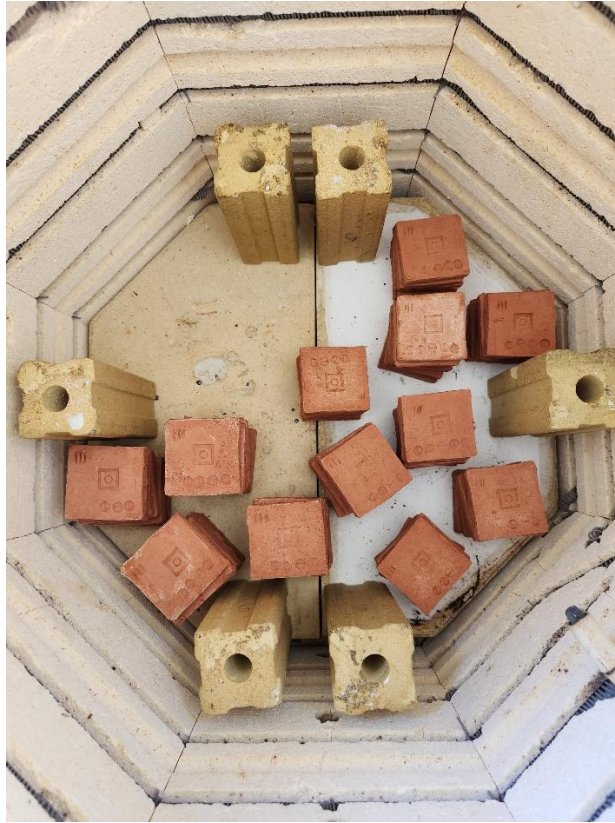
Figure 10 - Batch of tiles fired at 1000°C and ready to come out of the kiln
