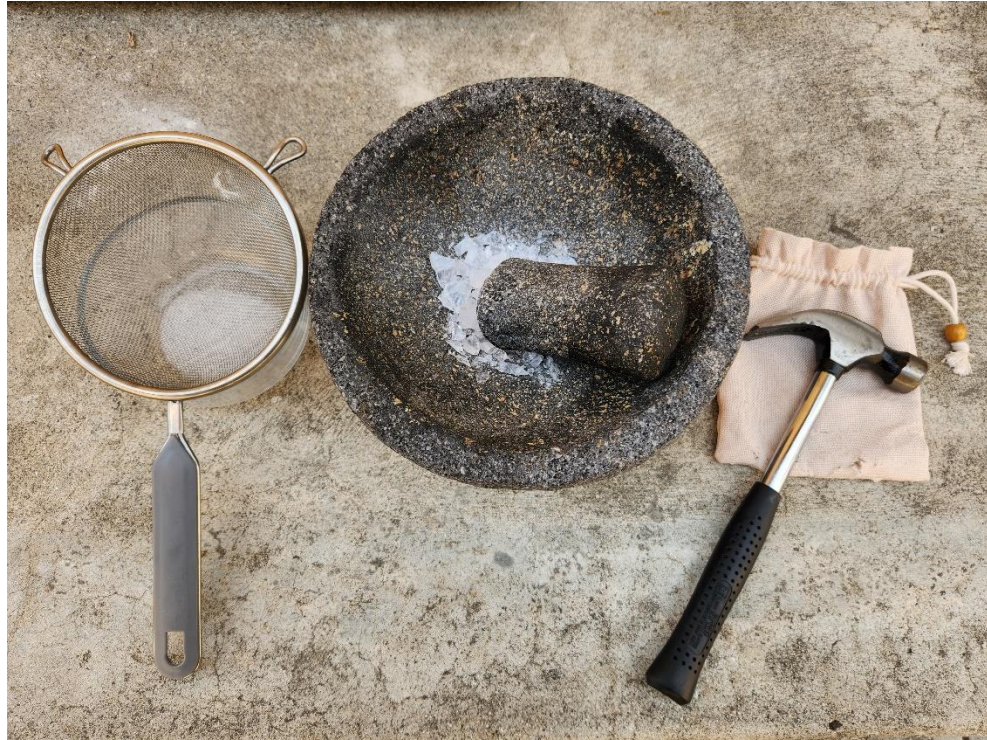
Figure 2 - Quartz being crushed for use as temper
