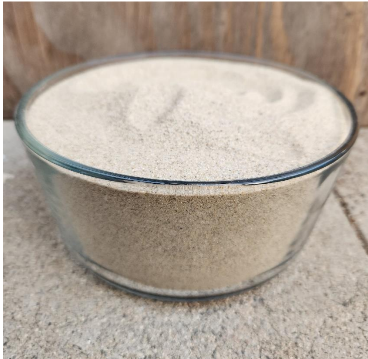
Figure 4 - Fine dune sand for use as temper
