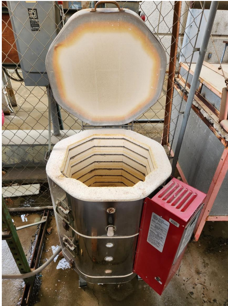
Figure 9 - One of the Skutt Model KM-822-3" electric kilns used to fire tiles
