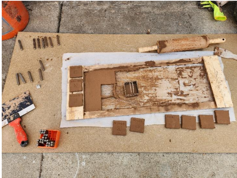
Figure 6 - Clay tiles being cut with molded die cutter
