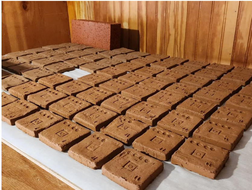
Figure 8 - Cut and coded tiles laid out to air-dry
