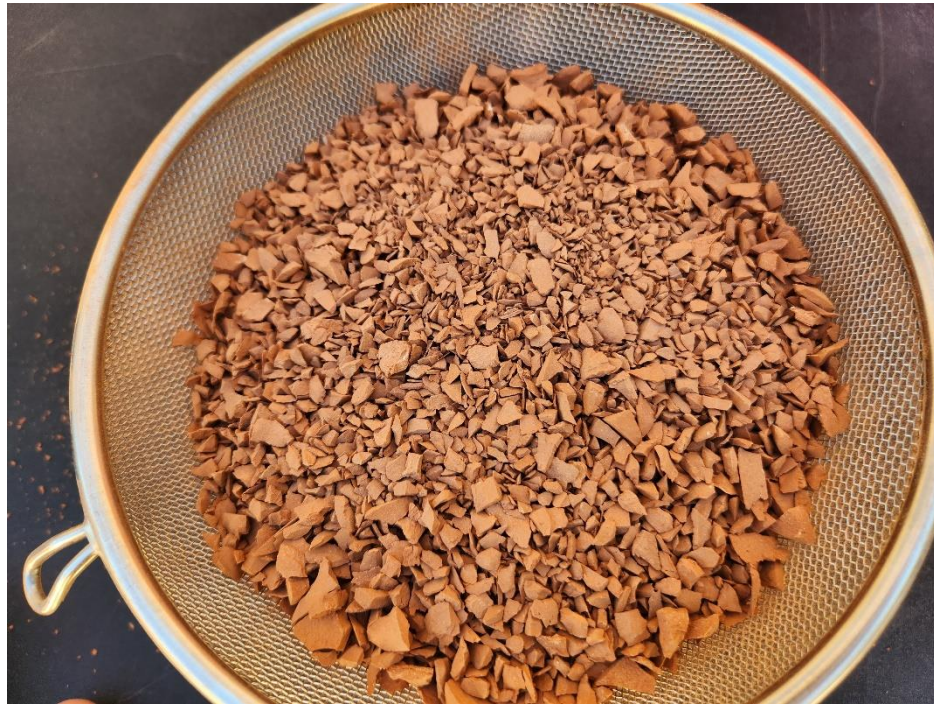
Figure 3 - Crushed ceramic (Grog) being strained for use as temper
