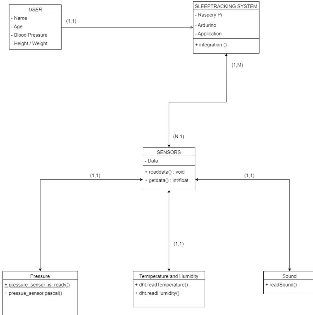
*Figure 9: Class Diagram*
