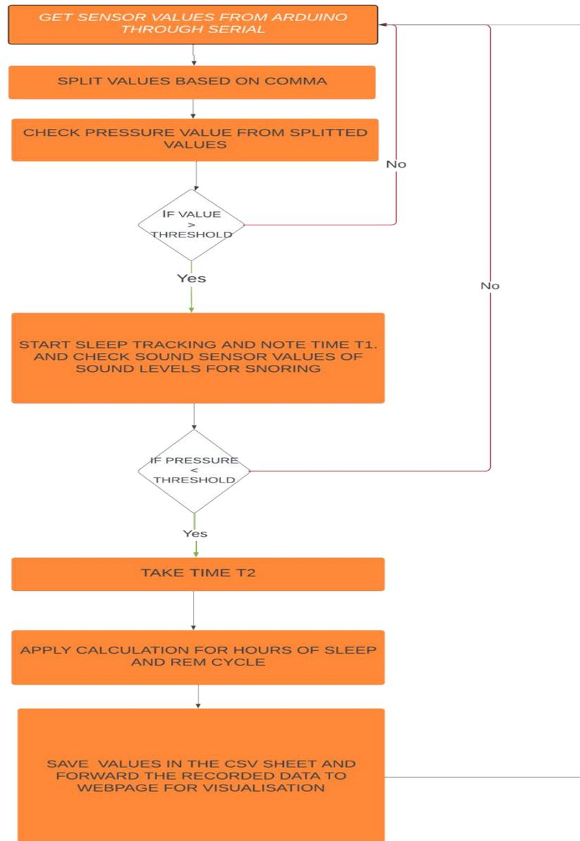
*Figure 6: Flow Diagram*
