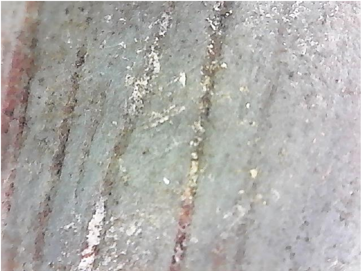
Figure 14. Example of Incision Variations. Photo by author under 100x magnification.
