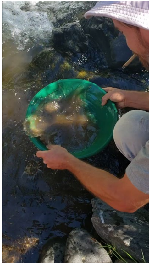
Figure 6. Showing a prospector separating gold from black sands using a gold pan. (Author's photo)
