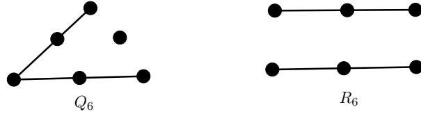
Figure 2.3: The matroids Q_6 and R_6 are the smallest examples of non-isomorphic matroids that have the same Tutte polynomial.
