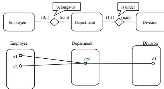
**Fig. 2 Database connections shown in an ER diagram**
