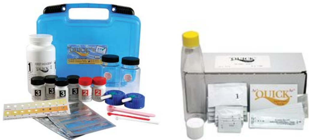
Figure 3. ITS Quick Rapid Arsenic Test Kit. Model number 481304 used for arsenic analysis of water and vegetation (left). Model number 481396-5 used for arsenic analysis of soil (right). Both test kits are EPA and ETV approved.
