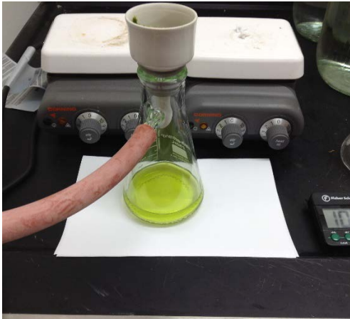
Figure 8. Alcohol extraction apparatus with ceramic Büchner funnel filter (CoorsTek 60239, 30mL) (left). Top view of Büchner funnel with vegetation sample (right).
