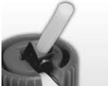
Figure 4. Turret Cap Used for Analysis of Arsenic in Both Water and Vegetation Samples.
