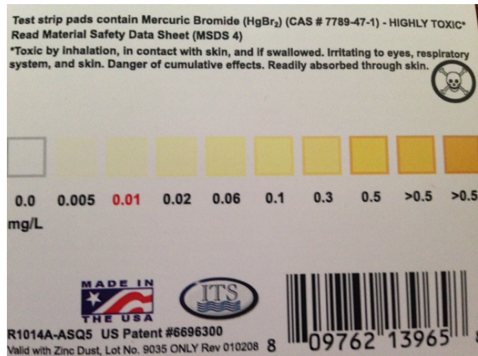
Figure 10. Color Chart for Arsenic Concentration in Soil Samples. Color match testing strip to color chart determines the amount of arsenic in sample.
