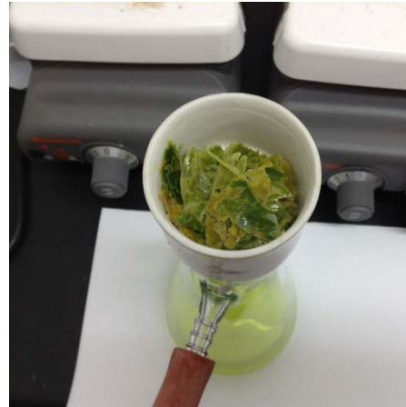
Figure 8. Alcohol extraction apparatus with ceramic Büchner funnel filter (CoorsTek 60239, 30mL) (left). Top view of Büchner funnel with vegetation sample (right).
