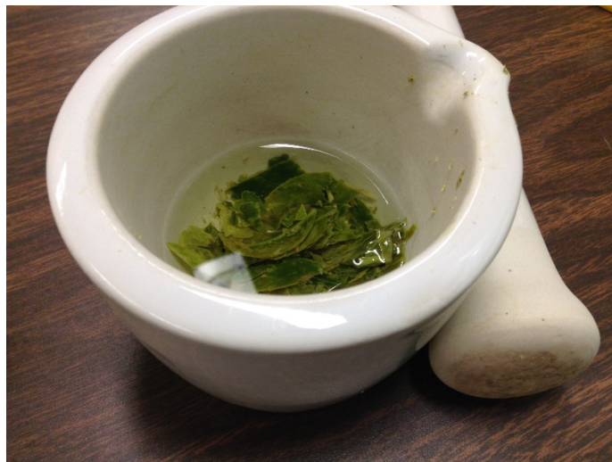
Figure 7. Mortar and Pestle with 50.0mL of Ethyl Alcohol and 2.0g of Vegetation Sample.
