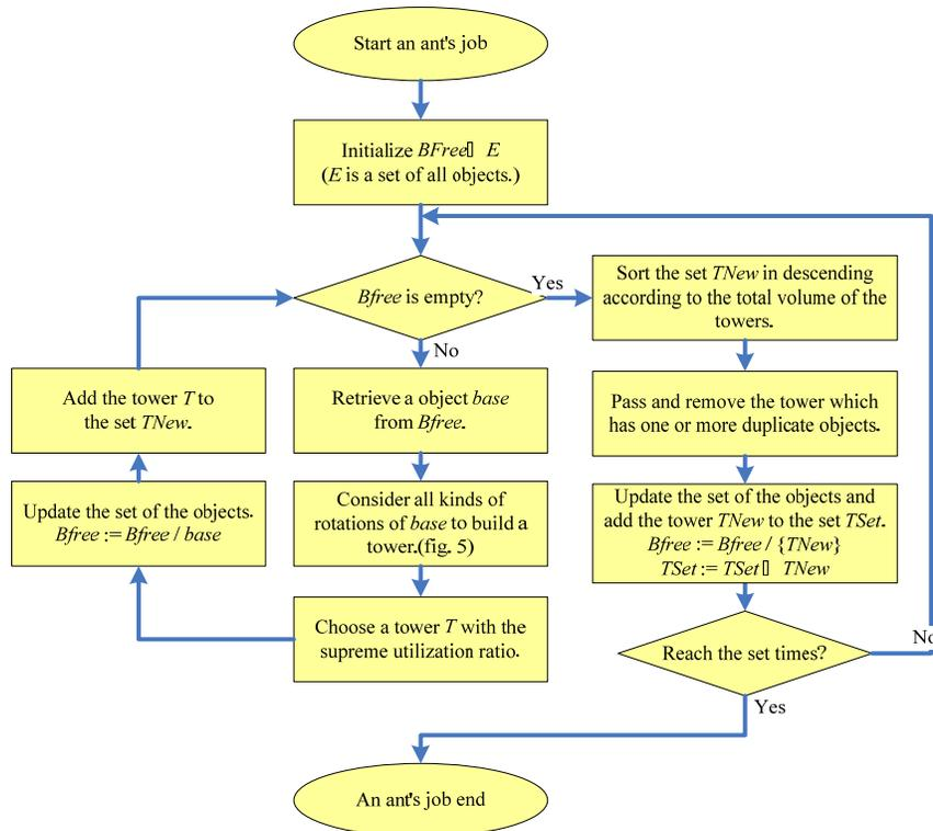
The procedure of constructing the tower is in a proper order, and incessant action of running too. The task of an ant is to choose the suitable objects and rotations to stack constantly. Then it feedbacks experience to the ants in the work or the ant of future generation, until one tower set is finished (The procedures are shown in figure 5 and figure 6).
