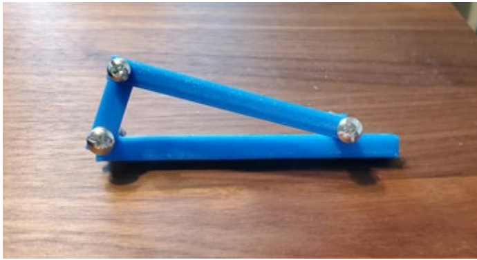
Figure 3. 3D Printed Slider-crank Mechanism
